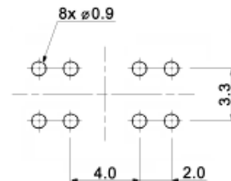
HOLE LAYOUT TOP VIEW \pm 0.05
